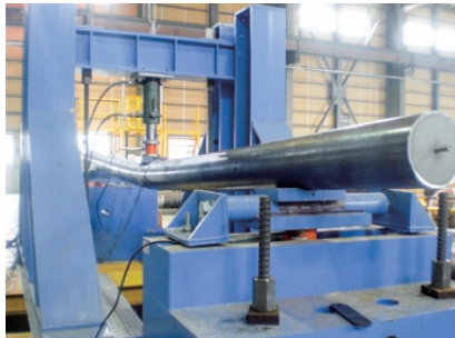
Loading test of static load to check bending moment of LST (Lotus-root Steel Tube)
